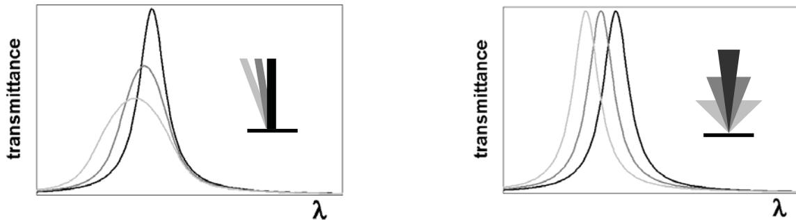
Fig 3: Influence of angle shift and divergence angle on bandwidth and peak transmittance of a FPF
