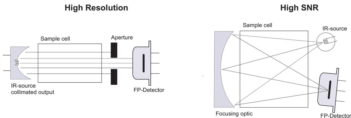
Fig 4: Possible optimizations for the optical design of a microspectrometer with FPF detector **left set up:** corresponds with an illumination by a parallel beam; **right set up:** corresponds with a high angle of incidence (AOI)
