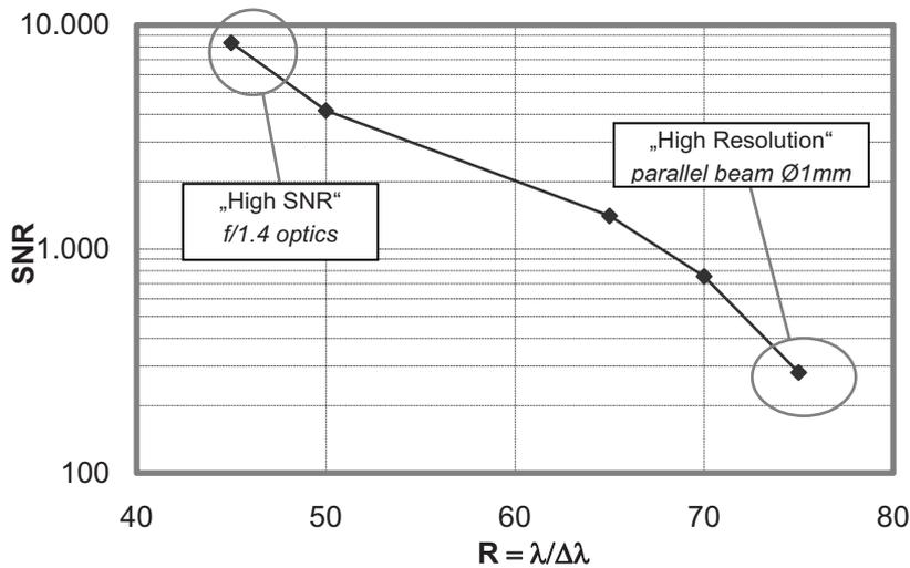
Fig 5: Measurements of the SNR vs. spectral resolution LFP-3041-337 with a modulated IR source at Hz, **left end point:** Illumination at high angle of incidence (AOI) using f/1.4 optics **right end point:** Illumination with a parallel beam ø 1 mm
