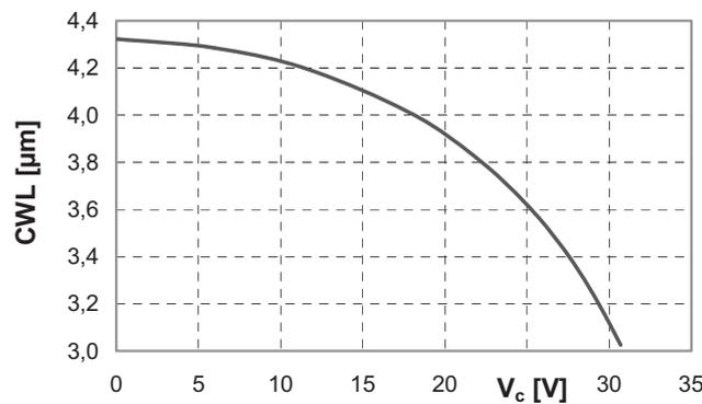
Fig 7: Typical steady-state control characteristic for LFP-3041L-337
