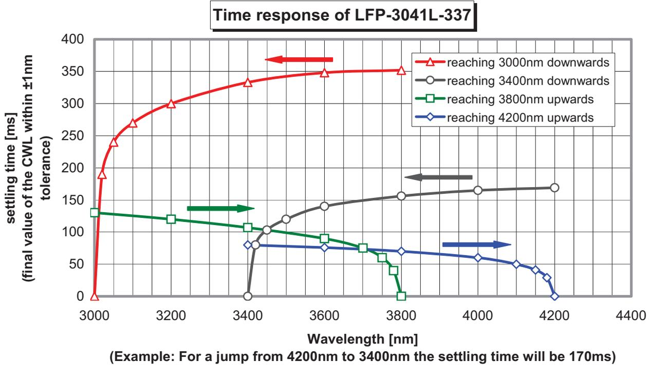
Fig 10: Transient response for LFP-3041L-337, typical values
