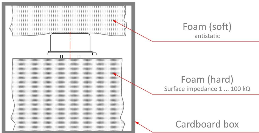
This packing is used for classic ESD protection. Otherwise, it also protects against inherent risks of pyroelectric detectors. A pyroelectric sensor element can generate a voltage of 1 kV if exposed to a temperature difference of some 10 K. In the case of an open connection configuration, which is often used for current mode detectors, high
